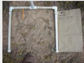
Figure 1. Enhanced Quadrat Frequency Frame (EFM), adopted from an existing quadrat frame, by the addition of 3 basal hit pins at the top and sides of the frame. The 10x10cm quadrat is in the upper left of the 40x40cm quadrat.
