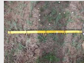
Figure 2. Point-Frequency Frame (PF) developed and used by Texas A&M University. It is comprised of five, 5x5cm quadrats equally spaced with a basal hit pin in the center of each quadrat.
