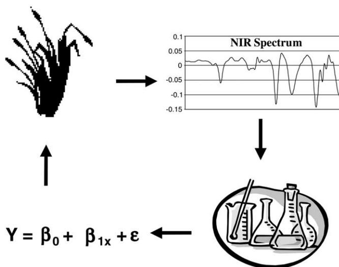
Fig. 1. Traditional direct method of applying NIRS is to analyze a particular product with both NIRS and traditional wet chemistry and pair this information in the calibration set to calculate a predictive equation. We can then use only the NIRS and bypass the need for wet chemistry. NIRS is usually faster, less expensive, and is non-destructive.
